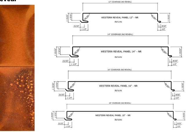
When the panels are installed side-by-side horizontally, the reveal forms a vertical gap between panels - making your project even more fascinating. Mix and match panels for a unique design.
