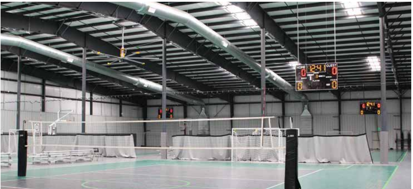
The Score OKC facility maintains a surplus level of light in summer, despite the small percentage of daylighting panels, saving energy.
